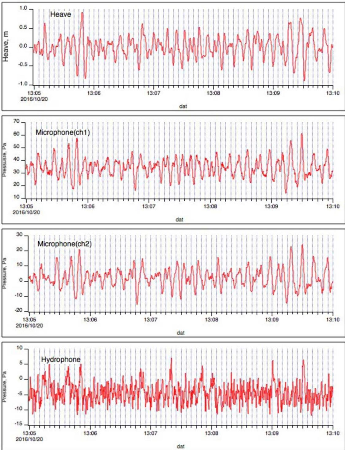
Figure 6: Simultaneous observation of heave (wave gauge), sonic waves (microphones 1 and 2), and underwater acoustic waves (hydrophone).
