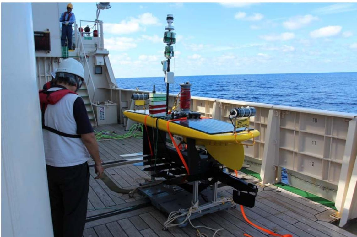
Figure 2: The wave glider about to be launched
