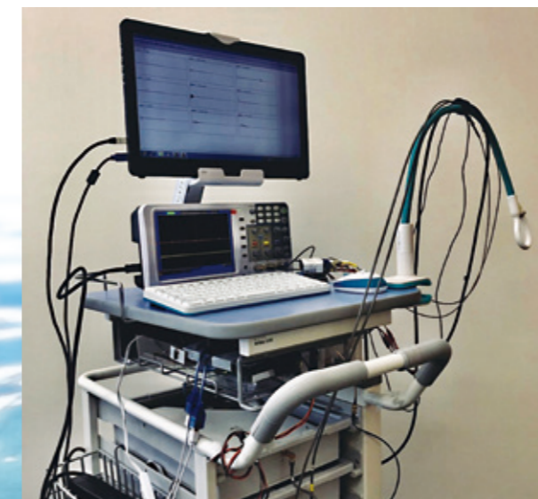
Screening using microwave mammography merely requires the antenna to be moved across the surface of the breast.
