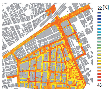
Thermal environment index at 13:00 on a sunny day in summer SET* distribution map (August 5, 2019)
