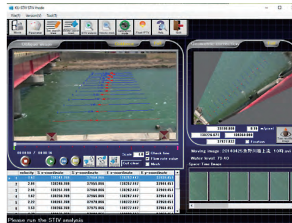
(Left) A screenshot of the KU-STIV software. “Searching lines” are superimposed on the river footage (top left), and flow speed is measured from the time taken for wave patterns and floating matter to cross these lines. Footage taken from the riverbank (from the side) is geometrically corrected into footage taken from above (top right), and velocity is calculated by analyzing the space-time image generated from the accumulation of individual wave patterns.
