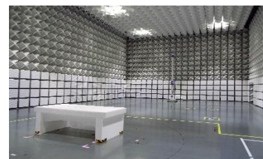
(10m法電波暗室)
